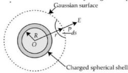
i. When point P lies outside the spherical shell: Suppose that we have to calculate electric field at the point P at a distance r (r > R) from its centre.
