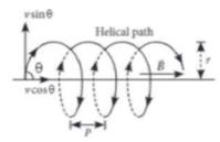
The plane of the circle is perpendicular to the magnetic field and the axis of the helix is parallel to the magnetic field. The charged particle moves along helical path touching the line parallel to the magnetic field passing through the starting point after each
