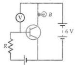
If the value of the resistance R is increased, the current in the forward-biased input circuit decreases. The emitter current IE decreases and hence the collector current ( $I_C = I_E - I_B$ ) also decreases. The glowness of the bulb decreases. Due to the decrease in I<sub>C</sub>, the potential drop across bulb B decreases, and hence the voltmeter shows a lower voltage.
